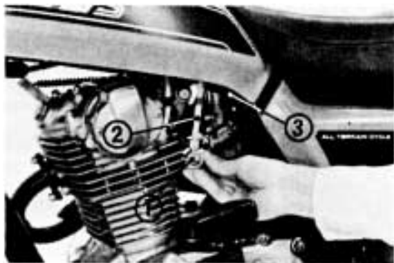
(1) Fuel valve (2) Fuel filter
