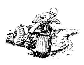
Incorrect turning technique may cause the front wheel to slide straight aheac when steered, without affecting the ATC's direction of travel. If this should occur, close the throttle, come to a stop, then continue practice, adhering to the technique out-lined on the preceding page.
