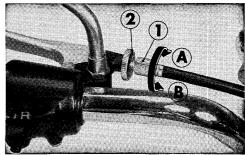
① Clutch cable adjuster bolt
