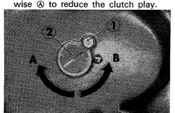
① Clutch adjuster locking bolt
