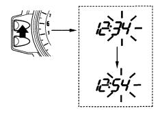
6. To end the adjustment, press control button B or turn the ignition switch OFF. The display will stop flashing automatically and the adjustment will be cancelled if the button is not pressed for about 30 seconds.
