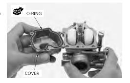
Install the float chamber cover and tighten the three screws.
