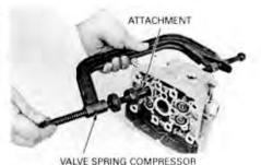
Loosen the valve spring compressor and remove the following:
