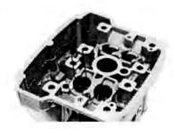
Check the valve lifter for scoring, scratches or damage. Measure the each valve lifter O.D.
