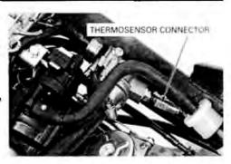
Turn the ignition switch ON and check the coolant temperarute gauge needle. The needle should move to "H".
