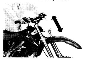
29. While keeping the forks parallel, alternately tighten the right axle pinch bolts (41) to the specified torque:
