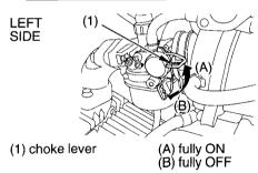
1. Pull the choke lever (1) up all the way to fully ON (A).
