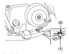
(1) oil drain bolt(2) sealing washer
