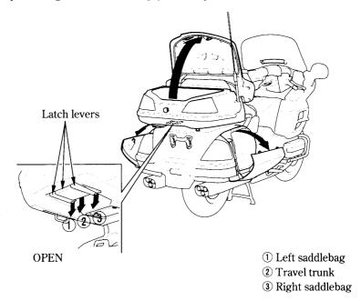
To shut each compartment, place your hands flat on the edges of its lid and press down until it is firmly closed and check the travel trunk & saddlebags open indicator is not displayed.
