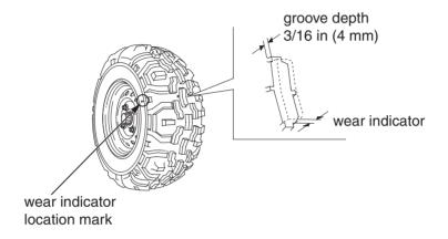
To check the condition of a tire tread, measure the groove depth in the center of the tire, or check the wear indicator.
