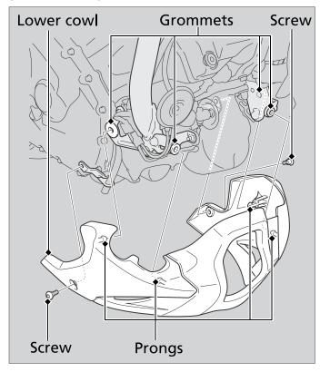
The lower cowl must be removed to service the coolant reserve tank, to replace the engine oil filter.
