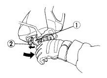
Make sure the throttle is closed and the rear brake is locked (page 33) before moving the motorcycle off the center stand.
