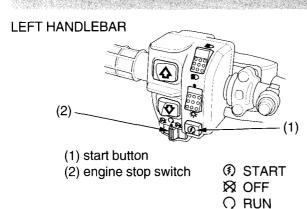
The start button (1) is used for starting the engine. Pushing the button in starts the engine. See Starting Procedure, page 57.
