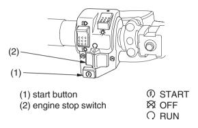
The start button (1) is used for starting the engine. Pushing the button in starts the engine. See *Starting Procedure*, page 55.
