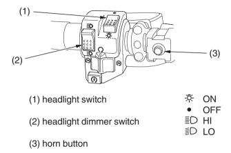
The headlight switch (1) is used to turn the headlight ON ( $\stackrel{*}{\sim}$ ) or OFF ( $\stackrel{\bullet}{\bullet}$ ). To operate, turn the switch to ON ( $\stackrel{*}{\sim}$ ) or OFF ( $\stackrel{\bullet}{\bullet}$ ).
