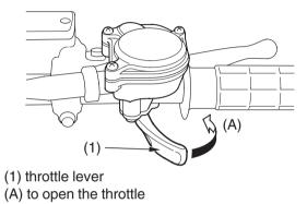
The throttle controls engine rpm (speed). To increase engine rpm, press the throttle lever (1) with your thumb. To reduce engine rpm, release pressure on the throttle lever. The throttle will automatically return to the closed position (engine idle) when you remove your thumb.
