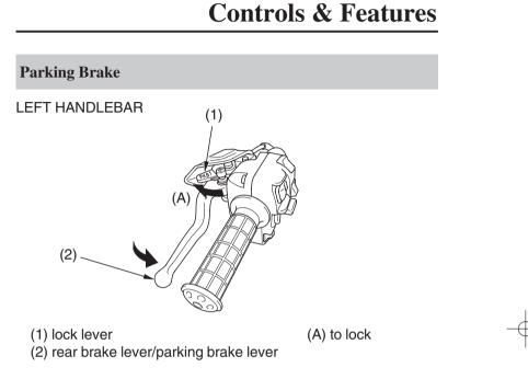
The lock lever (1) on the rear brake lever/parking brake lever (2) allows it to be used as a parking brake. To operate, first squeeze the rear brake lever/parking brake lever using your left hand and then lock it with the lock lever using your right hand. See *Parking* page 84.
