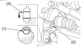
(1) oil drain plug(2) oil filler cap
