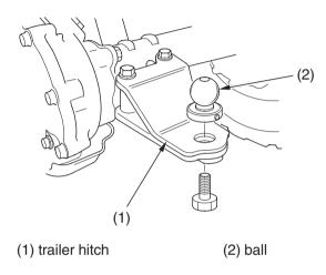
The trailer hitch (1) is located on the rear axle housing. To use the hitch, you'll need a proper size ball (2) as specified by the trailer manufacturer.
