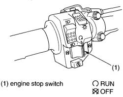
The engine stop switch (1) is used to stop the engine in an emergency. To operate, slide the switch to the OFF ( $\bowtie$ ) position. The switch must be in the RUN ( $\bigcirc$ ) position to start the engine, and it should normally remain in the RUN ( $\bigcirc$ ) position even when the engine is OFF.
