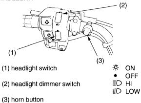
The headlight switch (1) is used to turn the headlight ON ( $\stackrel{*}{\times}$ ) or OFF ( $\stackrel{\bullet}{\bullet}$ ). To operate, turn the switch to ON ( $\stackrel{*}{\times}$ ) or OFF ( $\stackrel{\bullet}{\bullet}$ ).
