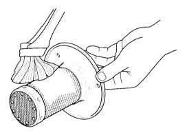
4. Install the spark arrester and the gasket in the muffler and tighten the three bolts securely.
