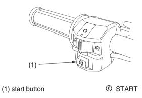
The start button (1) is used for starting the engine. Pushing the button in starts the engine. See *Starting Procedure*, page 56.
