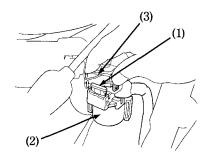
(1) Main fuse (3) Wire coupler (2) Starter magnetic switch
