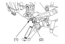
(1) engine oil (2) sealing washer drain bolt
