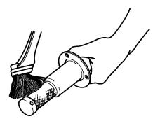
4. Install the spark arrester and the gasket in the muffler and tighten the three bolts securely.
