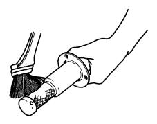
4. Install the spark arrester and the gasket in the muffler and tighten the three bolts securely.
