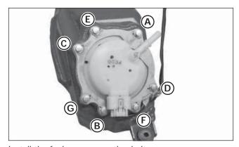
Install the fuel pump mounting bolts.
