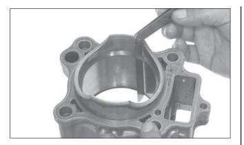
Insert each piston ring into the cylinder and measure the ring end gap.
