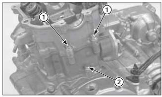
(1) CYLINDER HEAD BOLTS(2) CYLINDER SEALING BOLT
