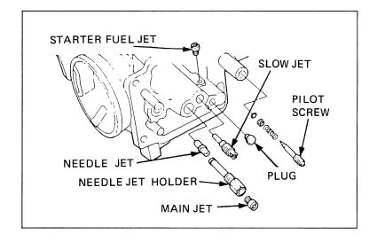
Remove the piston throttle valve (Page 4-11) and blow open all carburetor body openings with compressed air.
