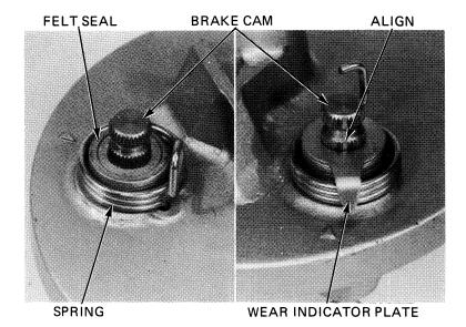
Install the brake arm, aligning the punch marks on the brake cam and arm.
