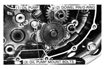
Remove the dowel pins and O-ring from the crankcase.
