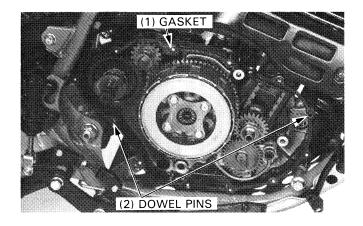
Turn the cam follower shaft arm clockwise to align the cam follower with the cam and install the right crankcase cover.
