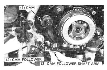
Tighten the cover bolts in a crisscross pattern in 2 or 3 steps.
