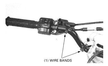
Place the front brake master cylinder on the handlebar and install the holder with the "UP" mark facing up.
