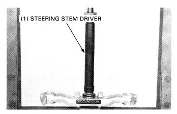
Drive new upper and lower ball races into the steering head pipe.
