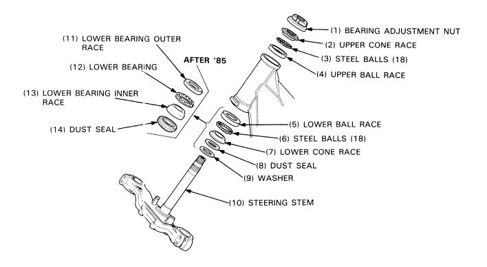
Install the washer and dust seal onto the steering stem and press a new lower cone race over the stem with the tool.
