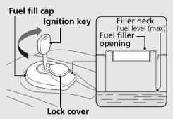
Do not fill with fuel above the plate. **Fuel type:** Unleaded gasoline only **Recommended fuel octane number:**Pump Octane Number (PON) 86 or higher. **Tank capacity:** 3.86 US gal (14.6 liters)
