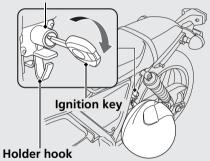
▶ Insert the ignition key and turn it clockwise to unlock. Hang your helmet on the holder hook. Turn the key counterclockwise to lock the holder hook and then remove the key.
