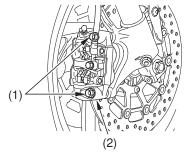
(1) fixing bolts(2) brake caliper assembly
