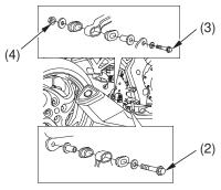
(2) muffler mount bolt A(3) muffler mount bolt B(4) muffler mount nut
