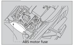
The ABS motor fuses are located on the starter magnetic switch.
