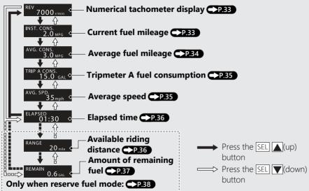
When the low fuel indicator lights and the low fuel pop-up information appear, INFO 3 display will automatically switches to the amount of remaining fuel display.
