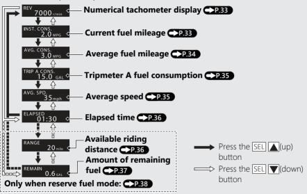
When the low fuel indicator lights and the low fuel pop-up information appear, INFO 3 display will automatically switches to the amount of remaining fuel display.
