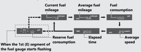
When the 1st (E) segment of the fuel gauge starts flashing, the current fuel mileage, average fuel mileage, fuel consumption, average speed or elapsed time switches to the reserve fuel consumption.
