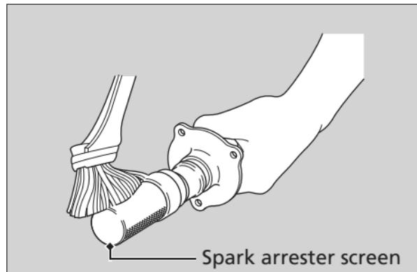
6. Install the gasket and the spark arresters, and tighten the bolts C.
