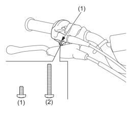
(1) M5×10 screw (2) M5×40 screw You can reduce throttle grip movement.
