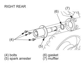
4. Remove the bolts (4), the spark arrester (5), and the gasket (6) from the muffler (7).
